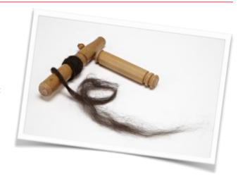
I had a couple of pieces of dowel that felt about right and cut them to size. For the pin, I used a coach bolt. I drilled a hole in the top of one piece and a larger hole through the other pin so that the bolt moved freely. To make mine spin a bit easier, I filed either side of the drilled hole on the horizontal to make it flat top and bottom. Then it was a simple matter of threading the bolt through the horizontal and fitting the bolt into the top of the other dowel.
