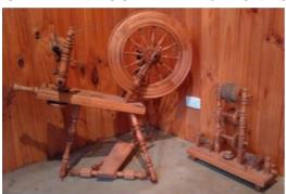
This Saxony spinning wheel was designed by Peter Tooth in 1992. Crafted from Canadian Rock Maple and finished with bees wax. Carefully looked after. Wheel diameter 460mm (18") and spindle orifice measures 10mm (3/8"). Ratios: options of 6:25, 8:5, 10:0, 12:4. Comes with six bobbins and Lazy Kate.
